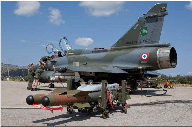
This EC03.003 Mirage 2000D is about to be loaded with two Raytheon GBU-22 Paveway III which is essentially a 500 lb MK 82 bomb with a Paveway III guidance kit. (652/133-XN, Souda, May 2011, Stephan de Bruijn)
