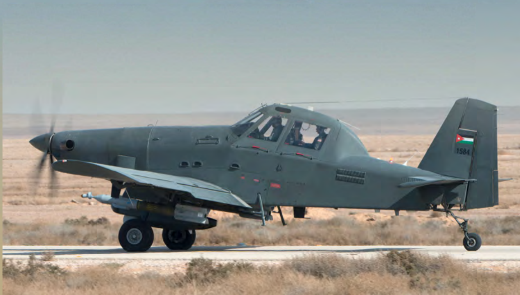
Above: Six former UAE AT-802 Air Tractors are now operating with the RJAF. The Block 1 configuration employs GBU-58 and GBU-12 Paveway II LGBs.
