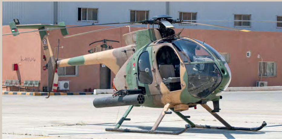
Above: Part of the Prince Hashim Royal Aviation Brigade, 28 Squadron operates eight MD530FF 'Little Birds' in the special operations role. Serial 2804 is armed with a seven-round 2.75in rocket launcher. Left: The RJAF training fleet has undergone a complete makeover and the Grob G 120TP has replaced the Slingsby Firefly in the basic training role. Fifteen are currently operated by 4 Squadron from King Hussein Air College/Mafraq.
